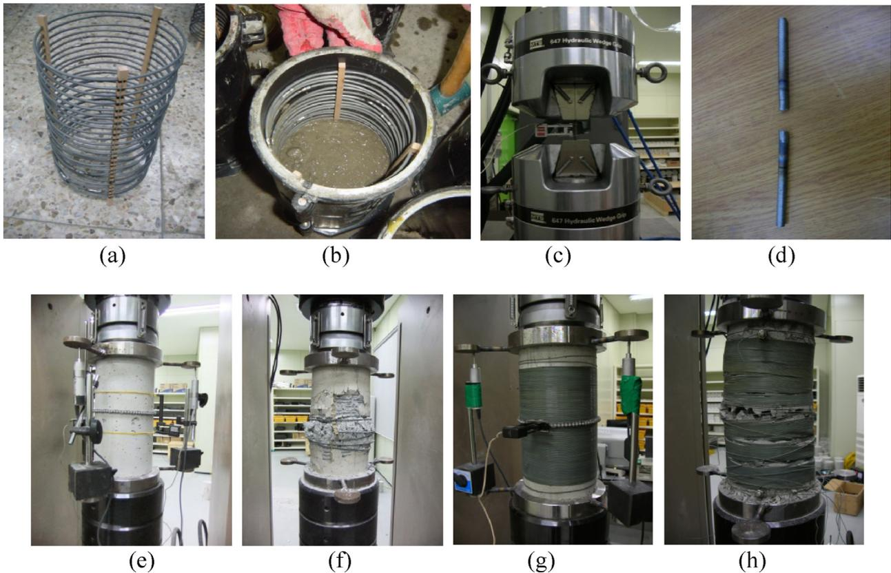
**Fig. 1.** (a) The suite of SMA rings. (b) SMA rings in a mold. (c) Tensile test of a welded SMA bar. (d) Fracture of a welded SMA bar. (e) Test set-up for a cylinder with SMA rings. (f) Failure of a cylinder with SMA rings. (g) Test set-up for a cylinder confined by a SMA wire jacket. (h) Failure of a SMA wire jacketed cylinder.
