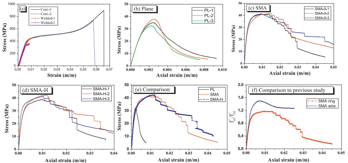
**Fig. 2.** (a) Tensile behavior of the welded SMA bars. Stress–strain curves of (b) plain concrete, (c) concrete confined by SMA rings, and (d) concrete confined by SMA rings with heating. (e) Comparison of the axial behavior of the three types of specimens. (f) Comparison to the results of a previous study.
