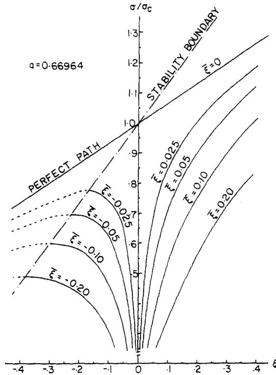
Fig. 1. Equilibrium paths of a single-mode asymmetric structural system ( $a = 0.66964$ ).
