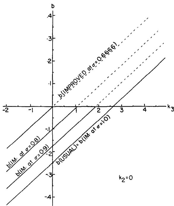
Fig. 2. The  $b$  (improved) coefficient vs the non-dimensional cubic spring constant for various values of the applied load ( $k_2 = 0$ ).
