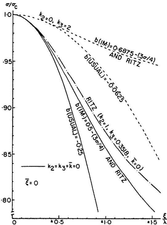
Fig. 4. Postbuckling paths of imperfect infinite beams using the  $b(\text{usual})$  and  $b(\text{improved})$  coefficients ( $k_2 = k_3 = 0$  and  $k_2 = 0, k_3 = 2$ ).
