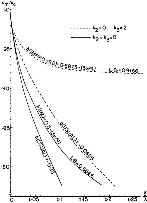
Fig. 3. The critical load vs the normalized imperfection amplitude using the  $b(\text{usual})$  and  $b(\text{improved})$  coefficients (for  $k_2 = k_3 = 0$  and  $k_2 = 0, k_3 = 2$ ).
