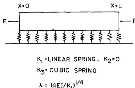
Fig. 1. A beam on a non-linear elastic foundation under axial compression.
