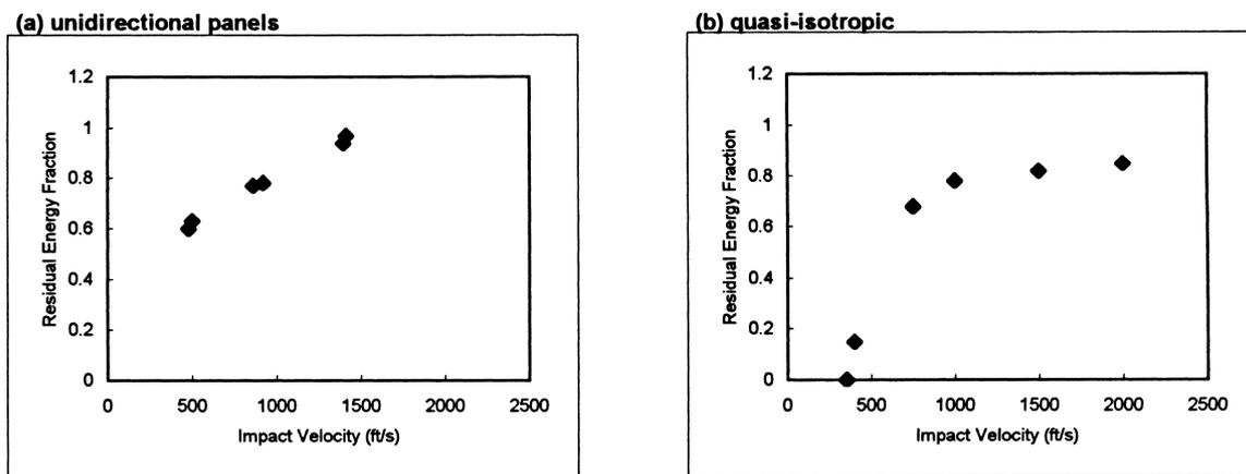
Fig. 7. Comparison of residual energy for the three targets. (a) Unidirectional Gr/Ep composite panels. (b) quasi-isotropic  $(0^\circ/22.5^\circ/45^\circ/67.5^\circ/90^\circ/-67.5^\circ/-45^\circ/-22.5^\circ)_2$ s graphite/epoxy panels.
