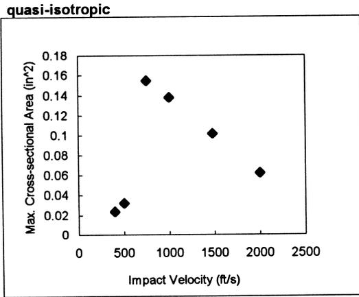
Fig. 8. Influence of impact velocity on shear plug size.
