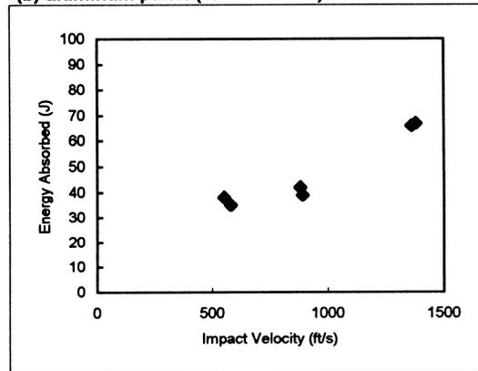
Fig. 5. (a) Energy absorbed by unidirectional Gr/Ep composite panels, (b) Energy absorbed by 1.27 mm (0.05 in.) thick 6061-T6 aluminum panels.
