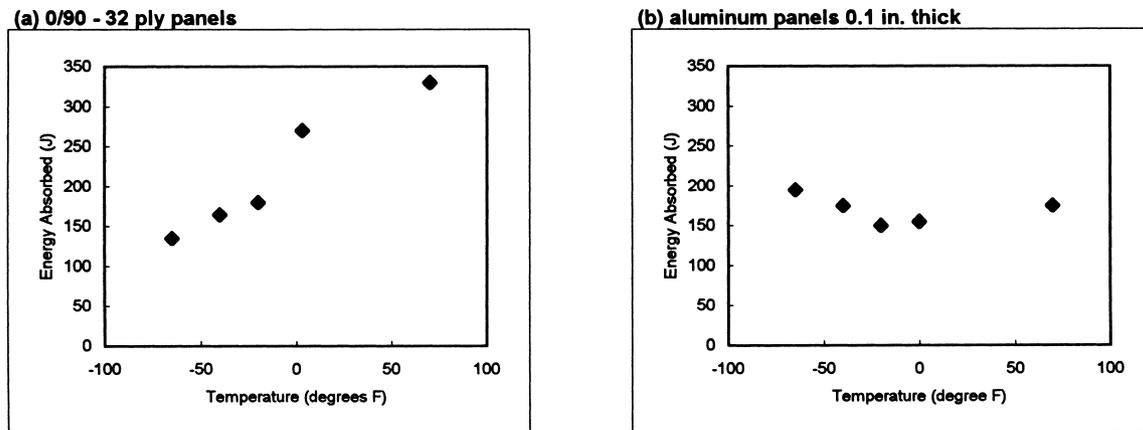
Fig. 6. (a) Energy absorbed by cross-ply Gr/Ep composite panels, (b) Energy absorbed by 2.54 mm (0.1 in.) thick 6061-T6 aluminum panels.
