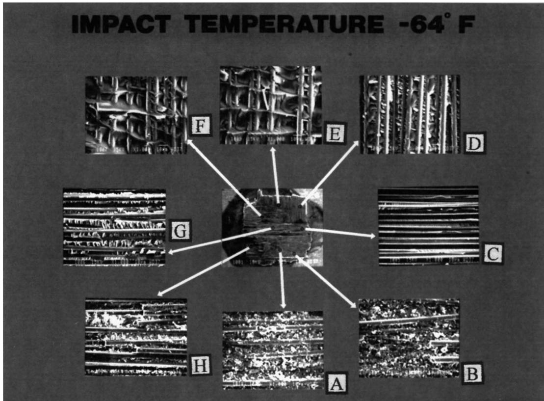
Fig. 10. Texture changes of micrographs with depth in shear plug at  $-53^{\circ}\text{C}$  ( $-64^{\circ}\text{F}$ ).
