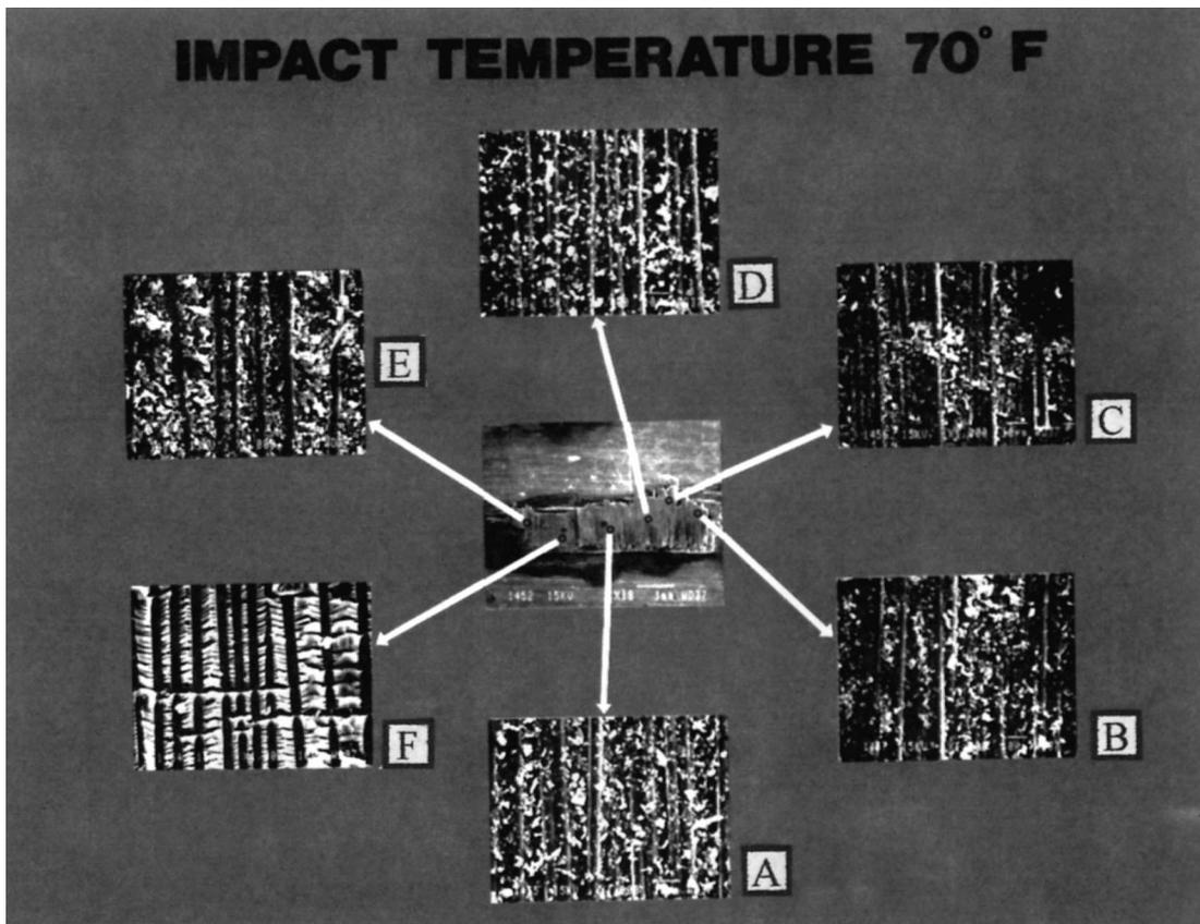
Fig. 9. Texture changes of micrographs with depth in shear plug at  $21^{\circ}\text{C}$  ( $70^{\circ}\text{F}$ ).
