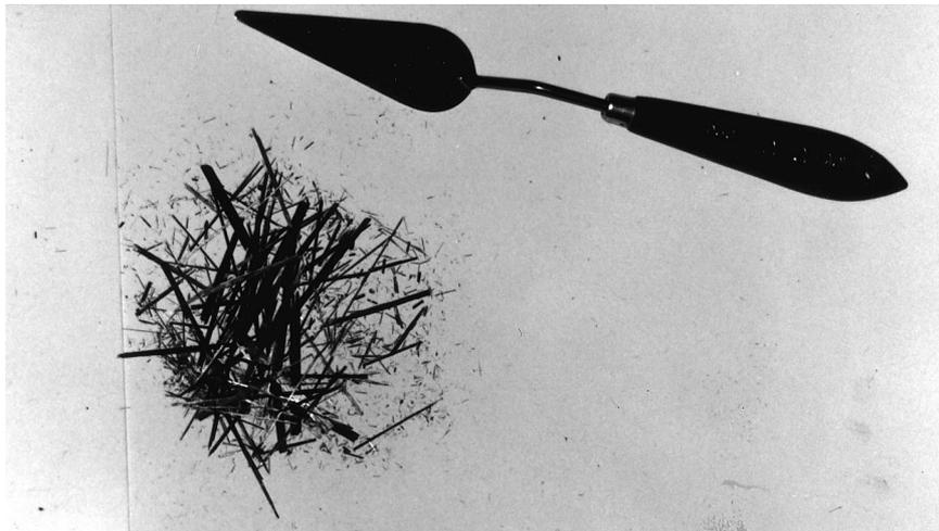
Fig. 3. Fragments collected from the rear side of a panel after impact.
