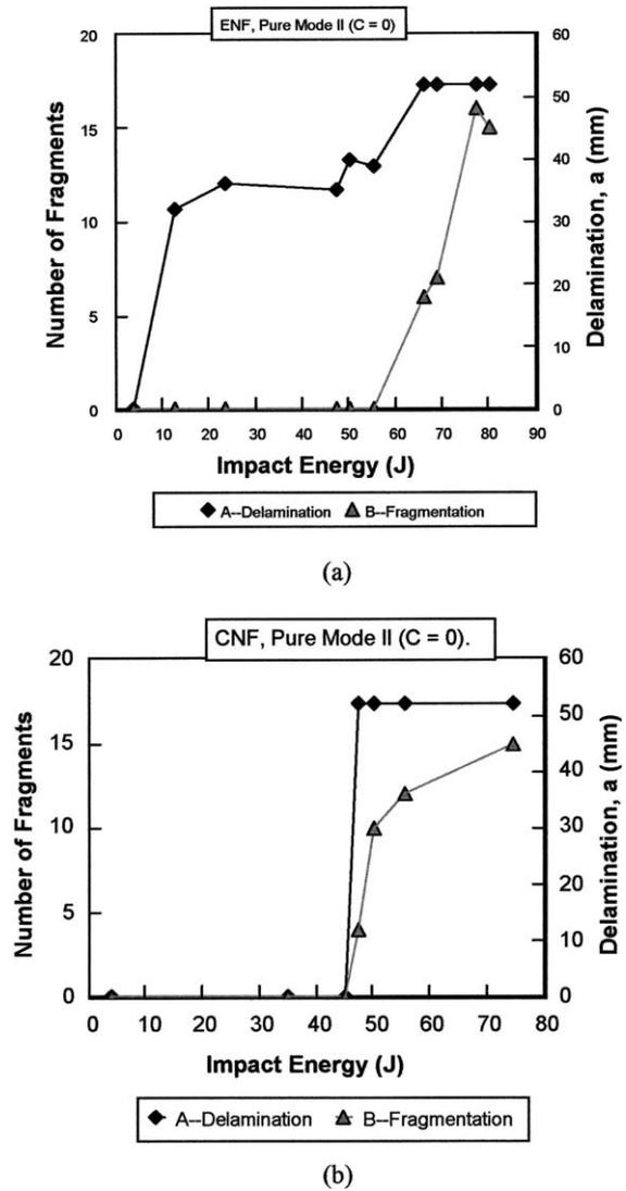
Fig. 7. Effect of impact energy on fragmentation for 24-ply (a) ENF and (b) CNF specimens.
