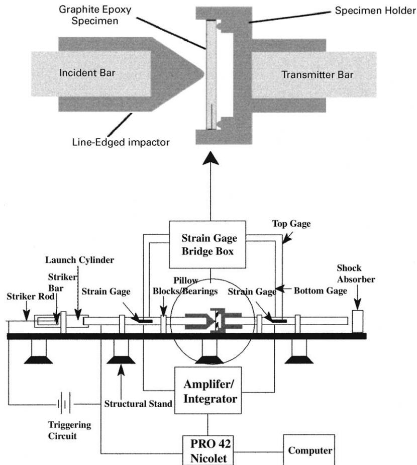
Fig. 1. Experimental set-up for dynamic mode II fracture test using ENF and CNF specimen and a fracturing split Hopkinson pressure bar.
