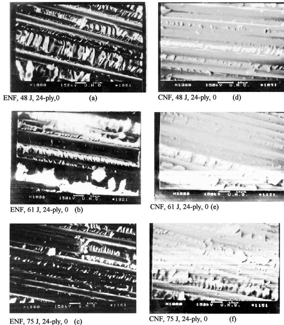
Fig. 10. SEM photographs of 24-ply for (a–c) ENF surfaces and (d–f) CNF surfaces near the end of insert at varying impact energy loaded at the center.
