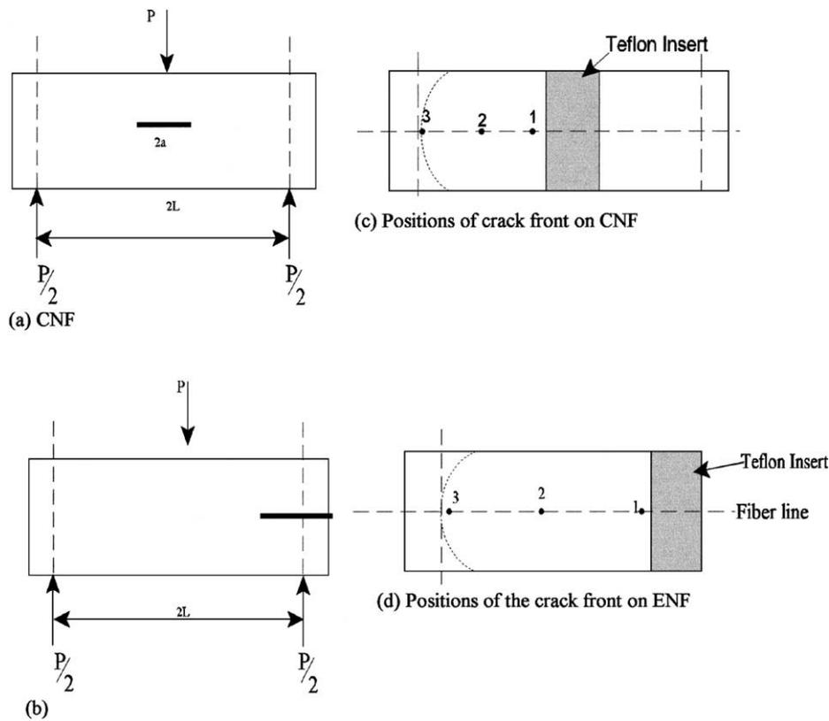
Fig. 2. Symmetrical loading and positions of the crack tip on the fracture surface for end-notch flexure (ENF specimen) and center-notch flexure testing (CNF specimen) for pure mode II fracture testing.
