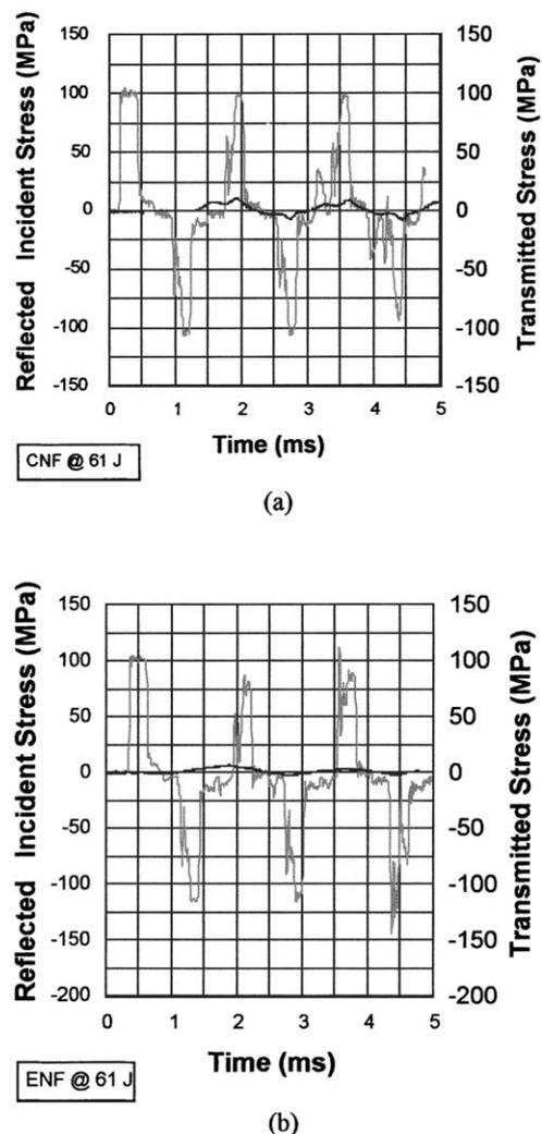
Fig. 3. Stress waveforms for pure mode II using 24-ply (a) CNF specimen and (b) ENF specimen.
