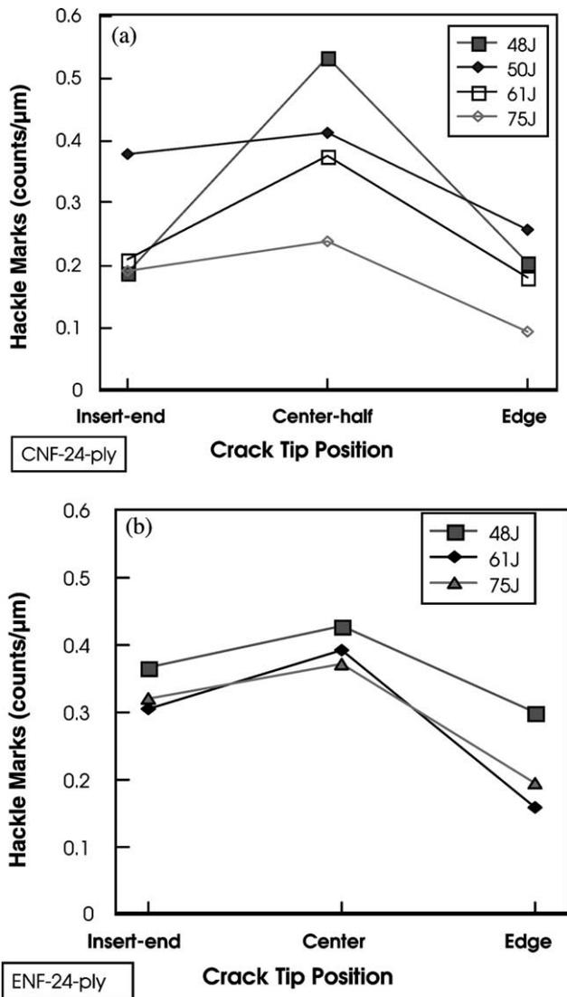
Fig. 12. Variation of hackle marks density with position of crack tip for 24 ply (a) CNF and (b) ENF specimens dynamically loaded at varying energies.
