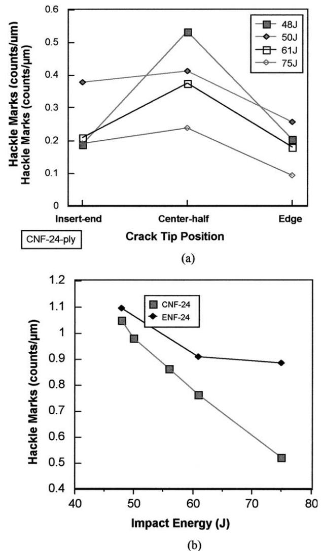
Fig. 11. Variation of hackle marks with loading energy for 24-ply ENF and CNF fracture surfaces.
