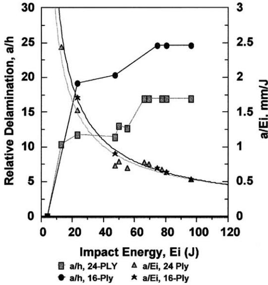
Fig. 6. Variation of thickness and energy normalized delamination with impact energy for ENF 16- and 24-ply specimens.
