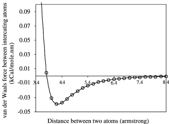
Fig. 5. Van der forces versus the distance between two carbon atoms.
