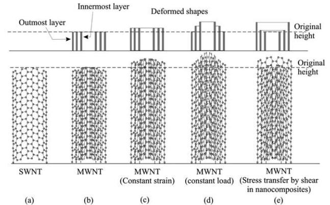
Fig. 7. Schematic illustration of the deformation shapes of nanotubes subjected to different load applications.
