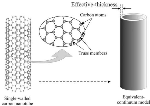
Fig. 4. Truss model of carbon nanotube's structure.
