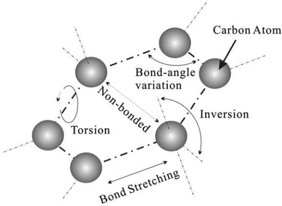
Fig. 2. Bond structures and corresponding energy terms of a graphene cell.
