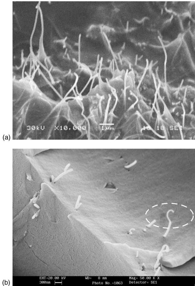
Fig. 6. Pull out of (a) the multi-walled carbon nanotubes and (b) an outermost layer of the nanotubes (right hand side).
