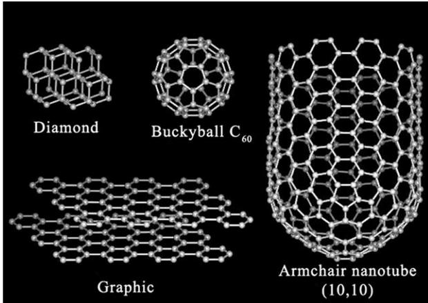
Fig. 1. Different forms of carbon-based materials.
