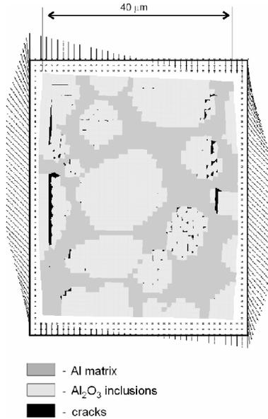
*Figure 4.* Mesocrack formation in the composite material with a matrix and brittle inclusions.
