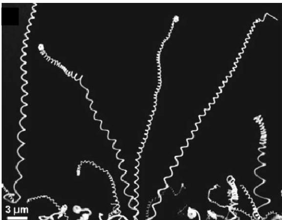
Fig. 7. SEM image of the coiled carbon nanotubes generated by pyrolysis of melamine over Co 'aged' catalytic substrates (in air).
