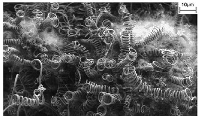
Fig. 13. SEM image of the micro-coiled carbon nano-fibres by template CVD.
