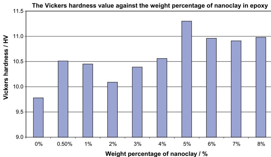
Fig. 4. The Vickers' hardness value of samples as a function of weight percentage of nanoclay in epoxy from 0 wt% to 8 wt%.
