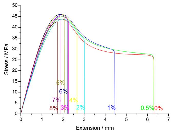
Fig. 2. The tensile curves of samples from 0 wt% to 8 wt% nanoclay, tested at a strain rate of 2 mm/min.
