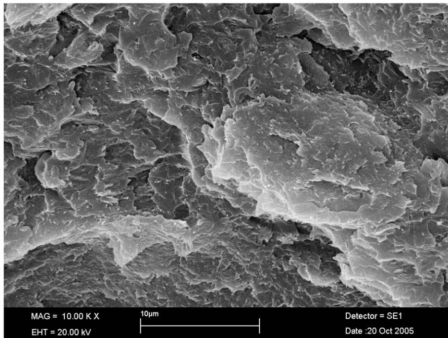
Fig. 10. The SEM image of 8 wt% nanoclay magnified in 10,000 $\times$ .
