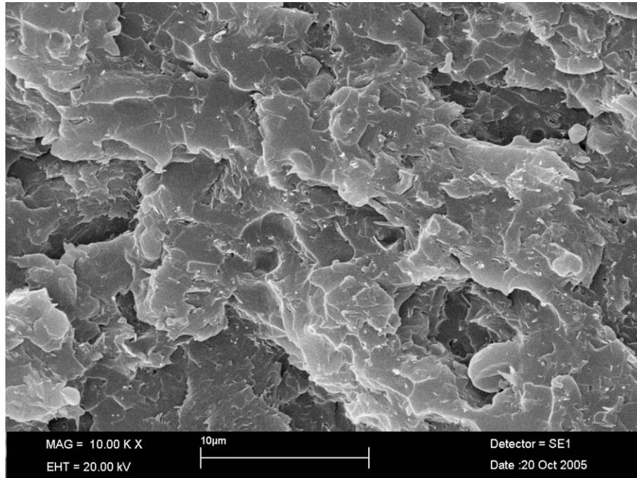
Fig. 9. The SEM image of 6 wt% nanoclay magnified in 10,000 $\times$ .
