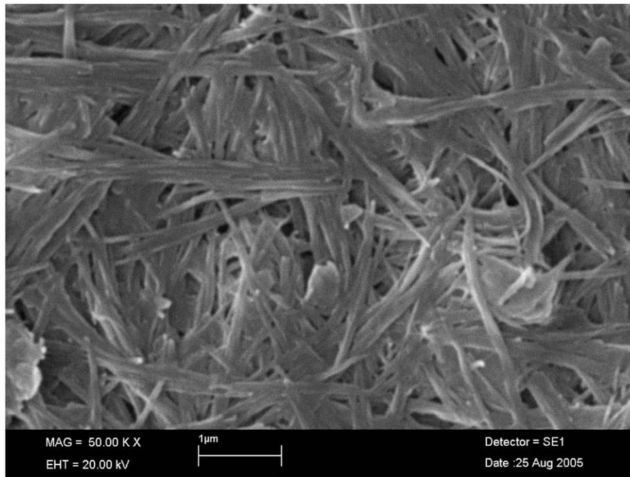
Fig. 5. The SEM image of nanoclay magnified in 50,000 $\times$ .
