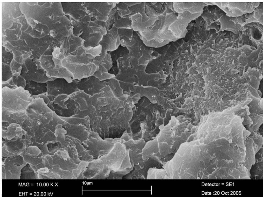
Fig. 8. The SEM image of 4 wt% nanoclay magnified in 10,000 $\times$ .
