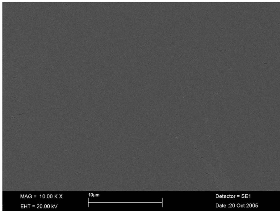
Fig. 6. The SEM image of pure epoxy (0 wt% nanoclay) magnified in 10,000 $\times$ .
