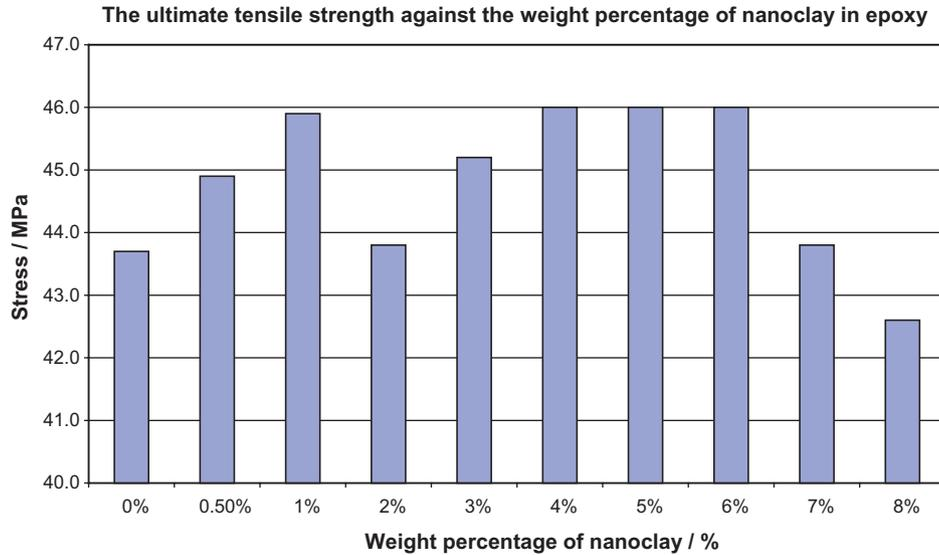
Fig. 3. The ultimate tensile strength of samples as a function of weight percentage of nanoclay in epoxy from 0 wt% to 8 wt%.
