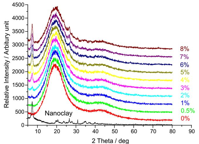
Fig. 1. XRD patterns of pure nanoclay and samples from 0 wt% to 8 wt%, scanned from 5° to 80° in  $2\theta$  scan.
