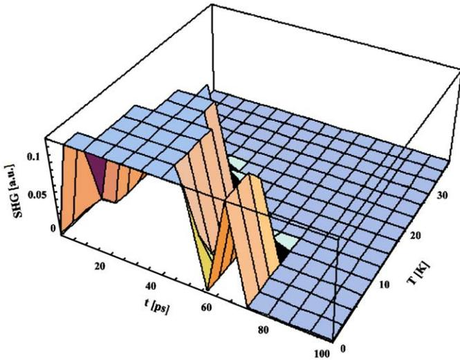
Fig. 3. Temperature dependence of the SHG for the InI nanocrystallites at different pump-probe delay time for the samples of the thickness 8 nm.
