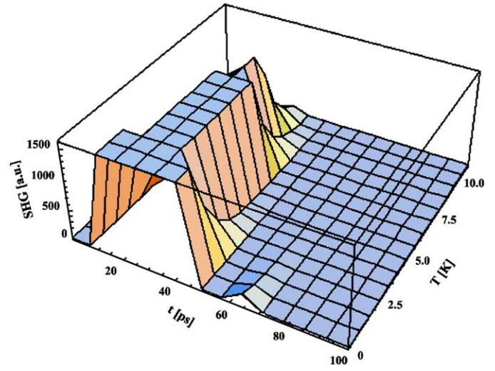
Fig. 5. Temperature dependence of the SHG for the InI nanocrystallites at different pump-probe delay time for the samples of the thickness 12 nm.
