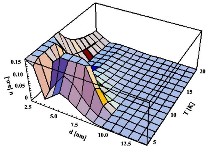
Fig. 6. Dependences of dilatometry measured relative deformation versus temperature and crystalline size.
