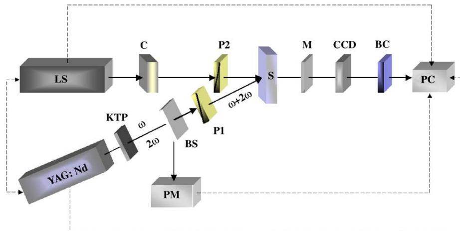
Fig. 1. Principal set-up for the measurements of the PISHG. YAG: Nd—pumping laser, LS—probing laser, C—chopper, BS—beam splitter, S—sample, M—monochromator, CCD—camera, BC—electronic boxcar, PC—personal computer, PM—photomultiplier, P1, P2—polarizers, KTP—crystal for double frequencies.
