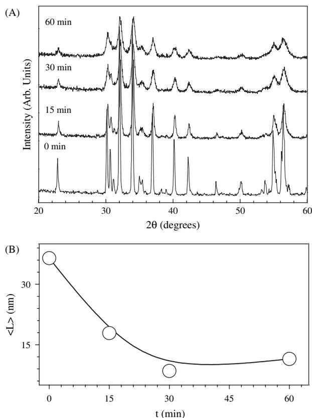
**Fig. 1.** (A) X-ray diffractograms of BaFe-SBS nanoparticles after different milling times. (B) The dependence of particle size on milling time, as estimated from the width of X-ray diffraction spectra (see Eq. (6)).
