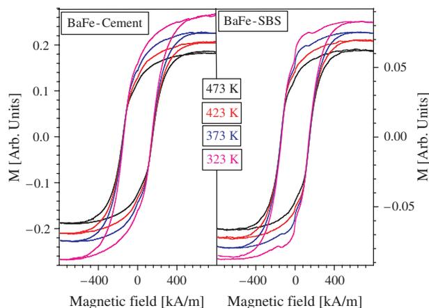
**Fig. 2.** The hysteresis loops of BaFe-SBS nanocomposites and BaFe-cement at various temperatures.
