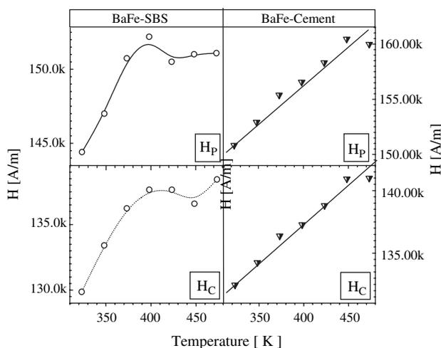
**Fig. 4.** The temperature dependence of the coercive field ( $H_C$ ) and of the peak field ( $H_p$ ).
