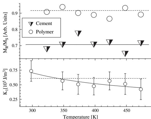
**Fig. 6.** Bottom panel: The temperature dependence of the magnetocrystalline anisotropy of BaFe in BaFe-SBS nanocomposites as estimated from Eq. (9). Upper panel: The temperature dependence of the squareness of hysteresis loops for BaFe-SBS and BaFe-cement.
