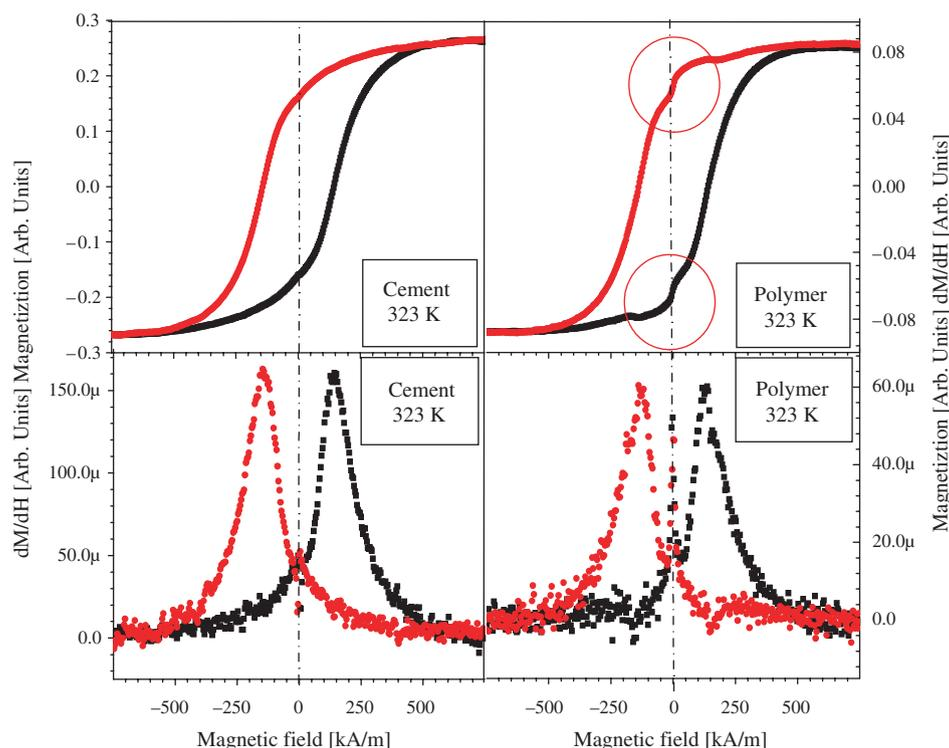
**Fig. 3.** The hysteresis loop of Ba-Fe cement (left panel) and BaFe-SBS at 50 °C. The upper panels show the hysteresis loops while the bottom panel shows the first derivative of the hysteresis loops relative to the magnetic field strength's.
