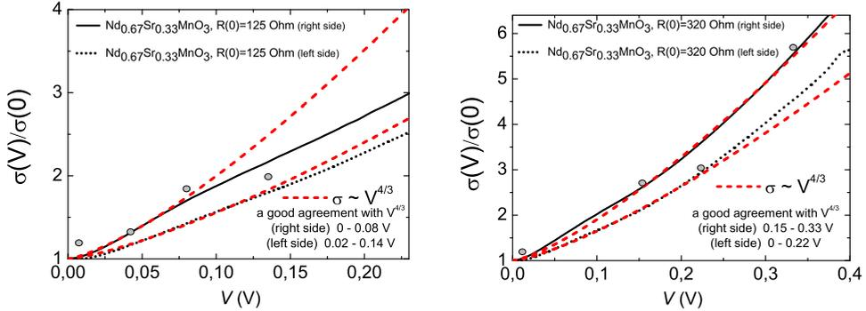
Fig. 2. Barrier characteristics of the Ag/NSMO junctions with the junction resistance  $R(0)$  equal to (a) 125  $\Omega$  and (b) 320  $\Omega$  for positive (solid line) and negative (dotted line) voltage signs. The dashed lines represent a conventional voltage dependence on the tunnel conductance predicted by the Glazman–Matveev model for an indirect tunneling. Arrows show voltage regions of the best agreement between the experiment and the theory. The temperature of the experiment was 77 K.
