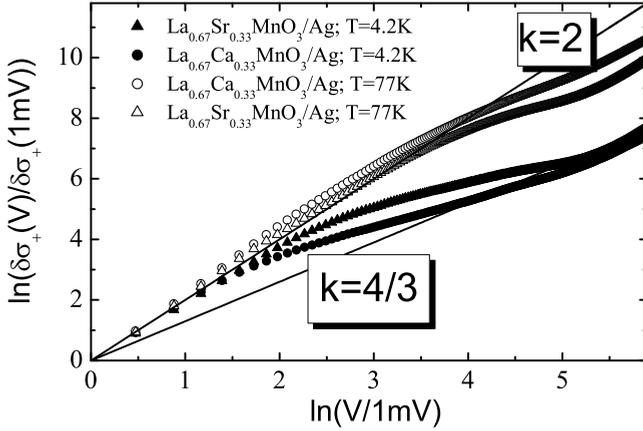
Fig. 3.  $\ln[\delta\sigma(V)/\delta\sigma(1\text{mV})]$  versus  $\ln(V/1\text{mV})$  dependence for the Ag/LSMO and Ag/LCMO junctions at 4.2 and 88 K. The straight lines correspond to a conventional elastic tunneling with  $k = 2$  and an inelastic tunneling through two metallic “drops” inside the potential barrier with  $k = 4/3$ .
