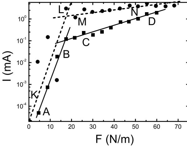
Fig. 5. An effect of increasing the force applied to a metallic tip on the tunneling current across a point contact formed between the tip and the LSMO surface. Squares and circles represent measurements for two different contacts at 0.5 V. Straight lines AB and KL indicate regions of a purely elastic deformation of the near-surface manganite layers whereas lines CD and MN correspond to the damage of the dielectric layer.
