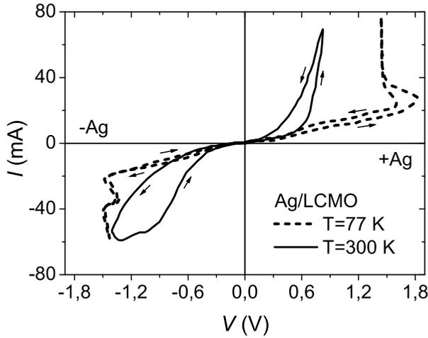
Fig. 4. An impact of high voltage biases applied to the Ag/LCMO junction at 77 and 300 R.
