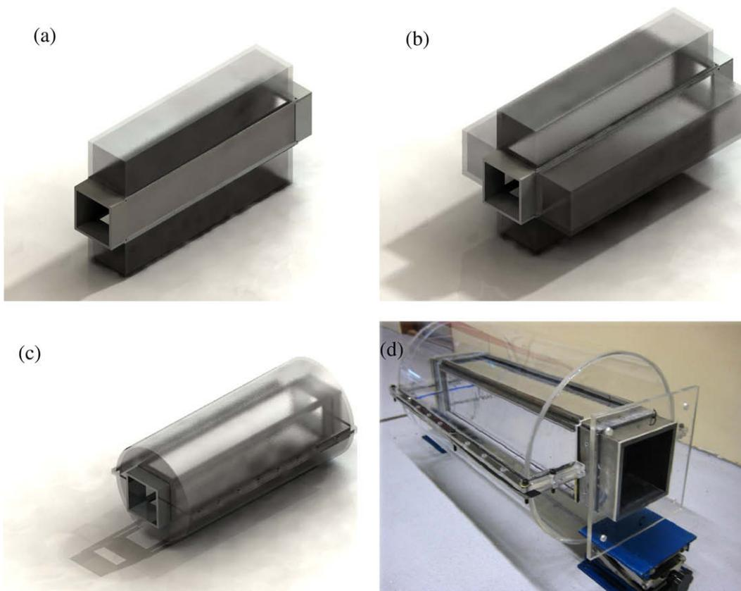
Fig. 11. (a) The model of 2-plate silencer, (b) is the model of 4-plate silencer with four rectangular chambers and (c) is the model of 4-plate silencer with cylindrical chamber and (d) is the prototype of 4-plate silencer.
