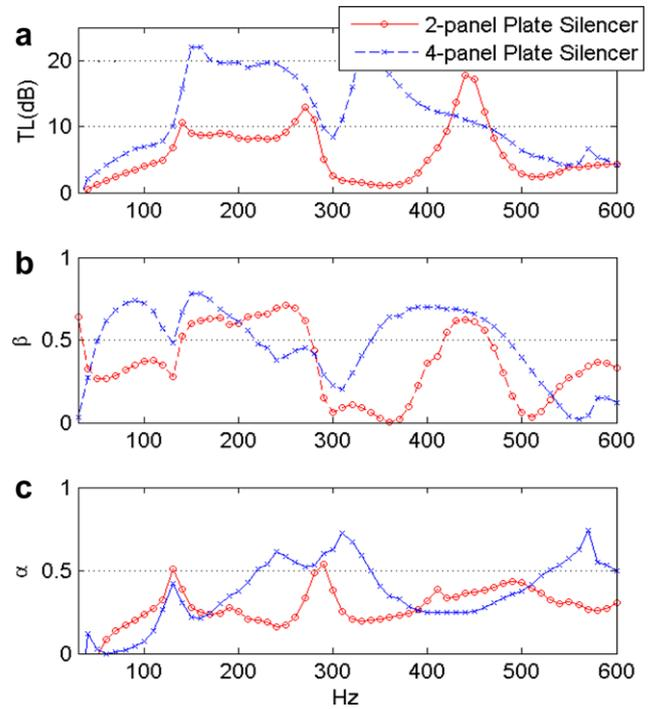
Fig. 12. Comparison between 2- and 4-panel plate silencer by using completely covered panel: (a) is the transmission loss, (b) is the reflection coefficient and (c) is the absorption coefficient.
