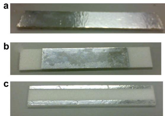
**Fig. 4.** The aluminum foil covered panels: (a) completely covered; (b) partially covered and (c) Zebra strip arrangement.
