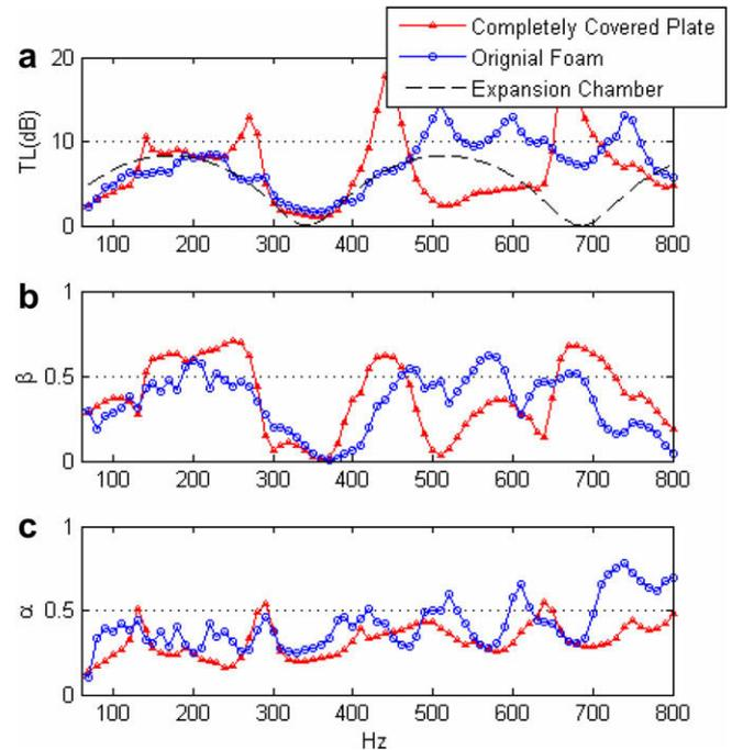
Fig. 8. Performance of the completely covered plate: (a) is the transmission loss, (b) is the reflection coefficient and (c) is the absorption coefficient.
