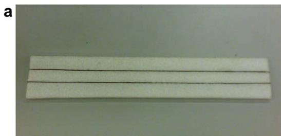
**Fig. 3.** The composite panel with two carbon fibre tows on the surface (a) is the configuration of the arrangement of the fibre tows on the plate, (b) and the result extracted from the flexural bending test.
