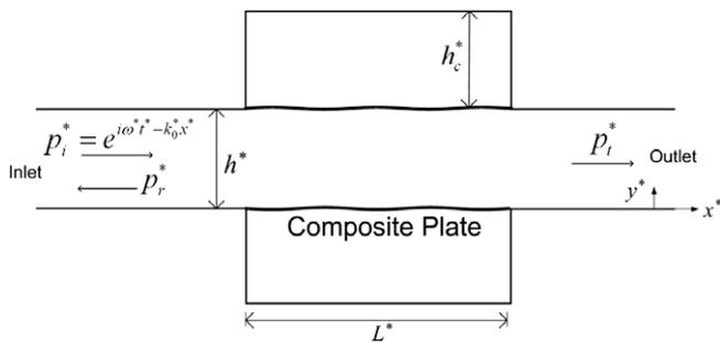
Fig. 1. Working principle of the plate silencer in two-dimensional configuration.
