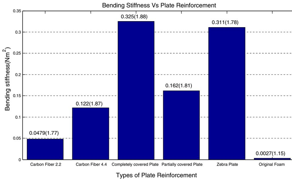
Fig. 5. Bending stiffness of six types of panel.
