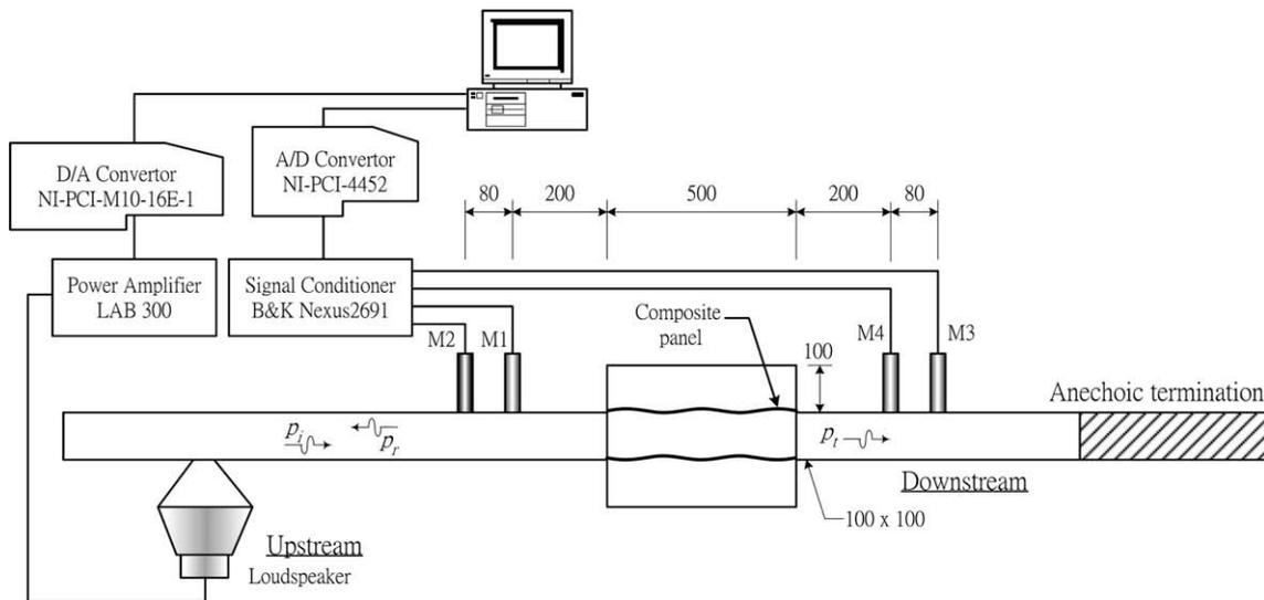
Fig. 6. Experimental set-up for transmission loss measurement.
