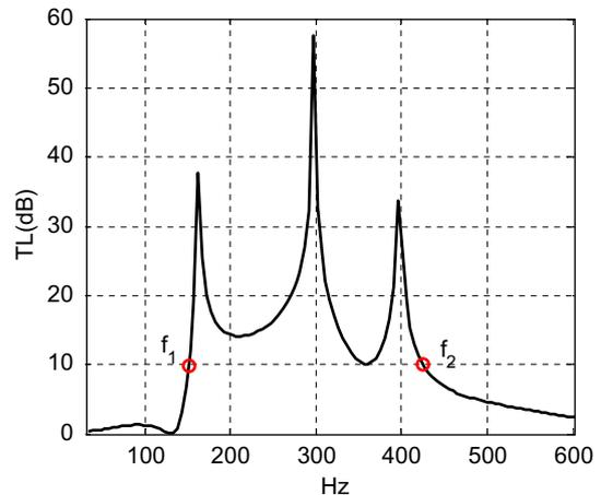
Fig. 2. Transmission loss spectrum for the plate silencer when  $m = 1$  and  $B = 0.0698$ .
