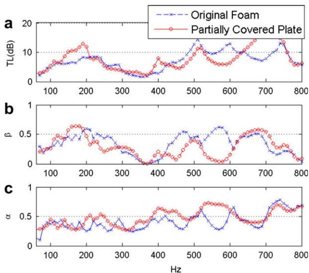
Fig. 9. Performance of the partially covered panel: (a) is the transmission loss, (b) is the reflection coefficient and (c) is the absorption coefficient.
