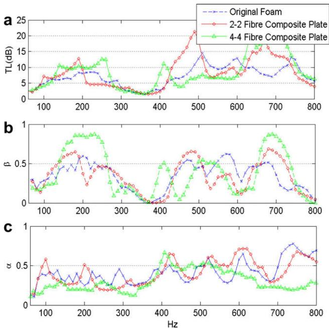
Fig. 7. Comparison between original foam, 2-2 carbon fibre and 4-4 carbon fibre composite plate (a) is the transmission loss, (b) is the reflection coefficient and (c) is the absorption coefficient.
