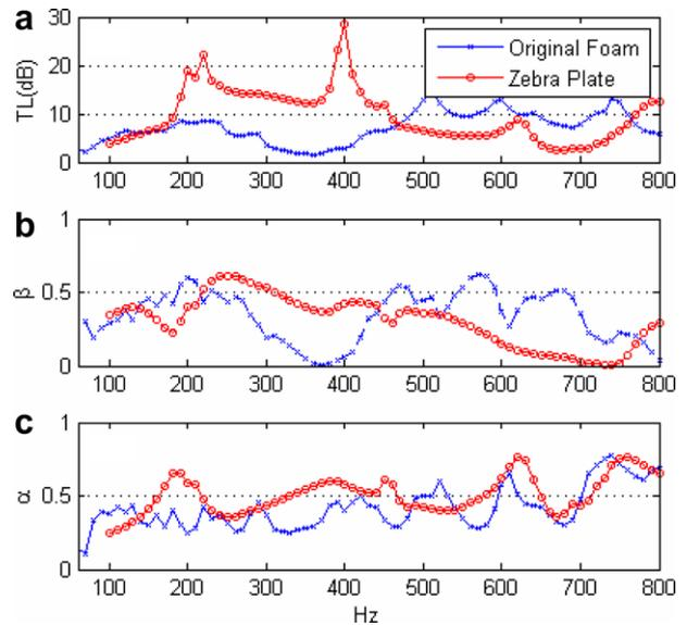
Fig. 10. Aluminum reinforcement – Zebra plate (a) is the transmission loss, (b) is the reflection coefficient and (c) is the absorption coefficient.
