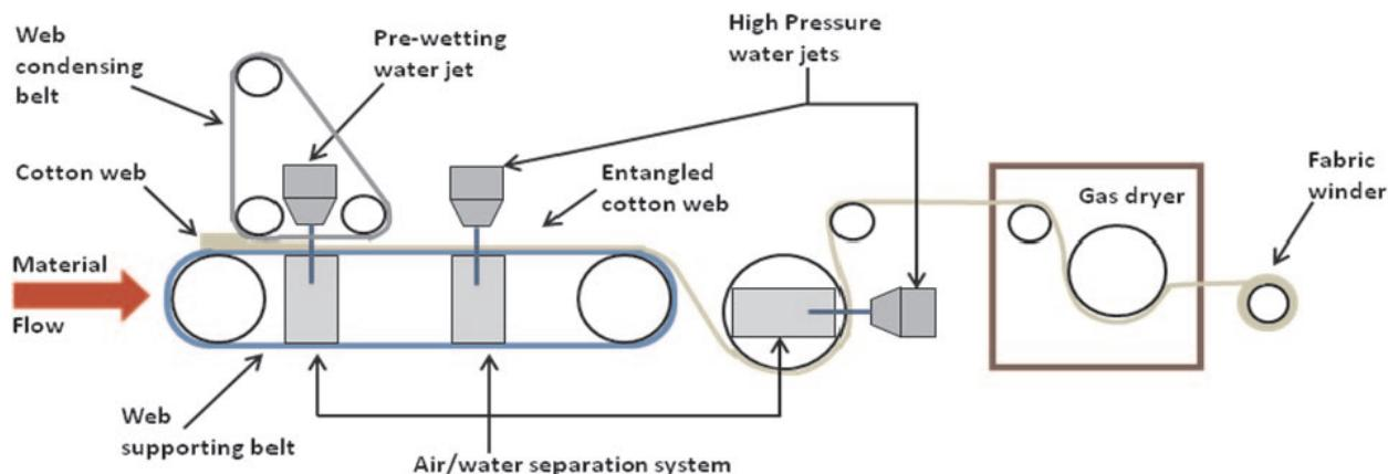
Figure 1 Schematic diagram of the commercial hydro-entanglement process used in the study.
