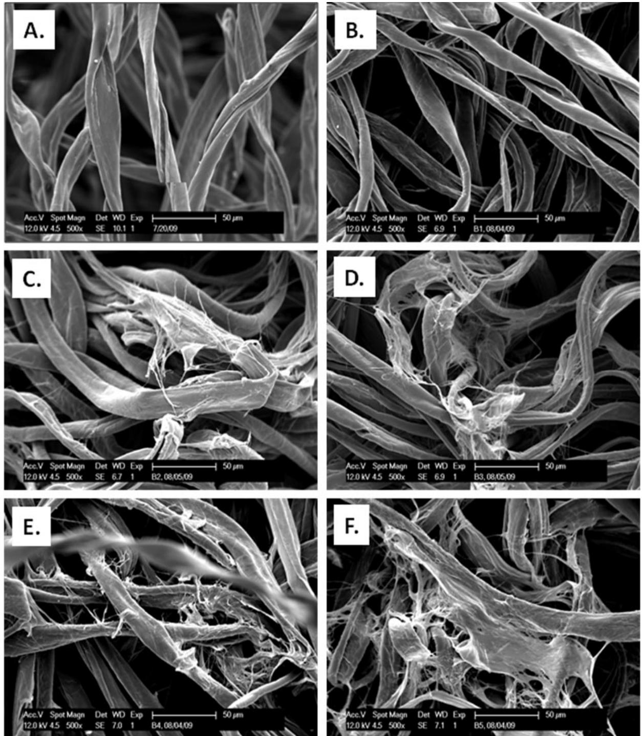
**Figure 4** SEM images of the hydro-entangled, greige-cotton non-woven fabrics produced at a constant pre-wetting pressure of 50 bar and the entanglement (HP) pressures ranging from 50 to 200 bar: (A) only carded cotton web; (B) 50 bar; (C) 75 bar; (D) 100 bar; (E) 150 bar; and (F) 200 bar.
