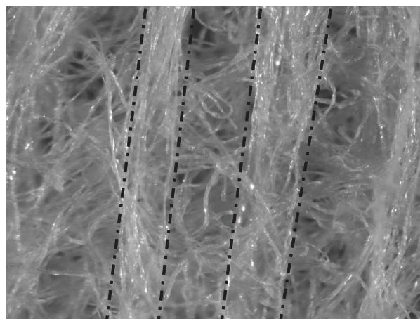
**Figure 3** Well-defined “strands” (denoted by the dashed lines) of fibers as observed in the machine direction.
