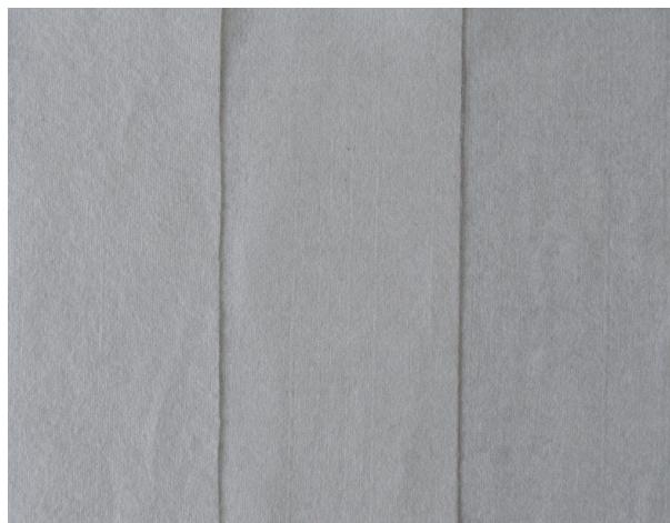
Figure 2 Appearance uniformity of a greige cotton non-woven fabric made by hydro-entanglement process.
