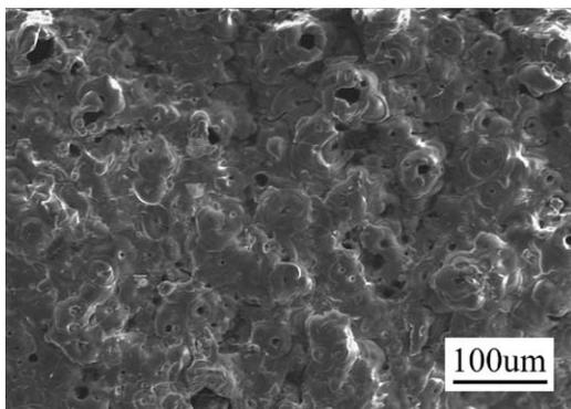
Fig. 2. SEM photograph of the MAO coating.
