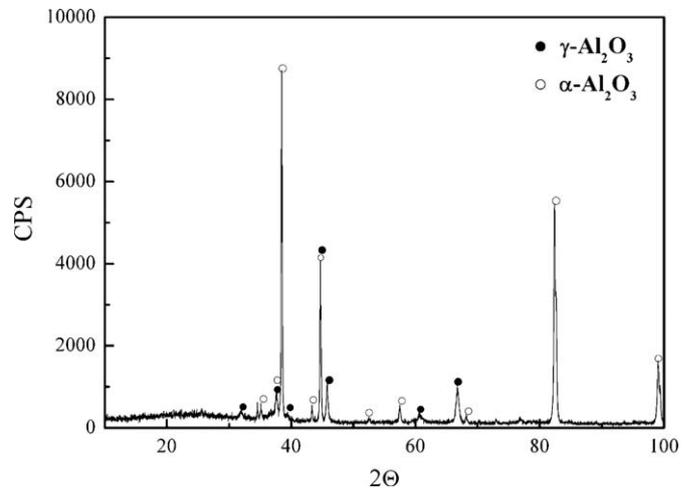
Fig. 3. XRD spectrum of the MAO coating after polishing.
