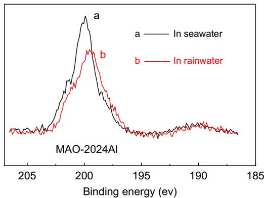
Fig. 11. XPS spectra of the wear scars in corrosion media (Cl<sub>2p</sub>).
