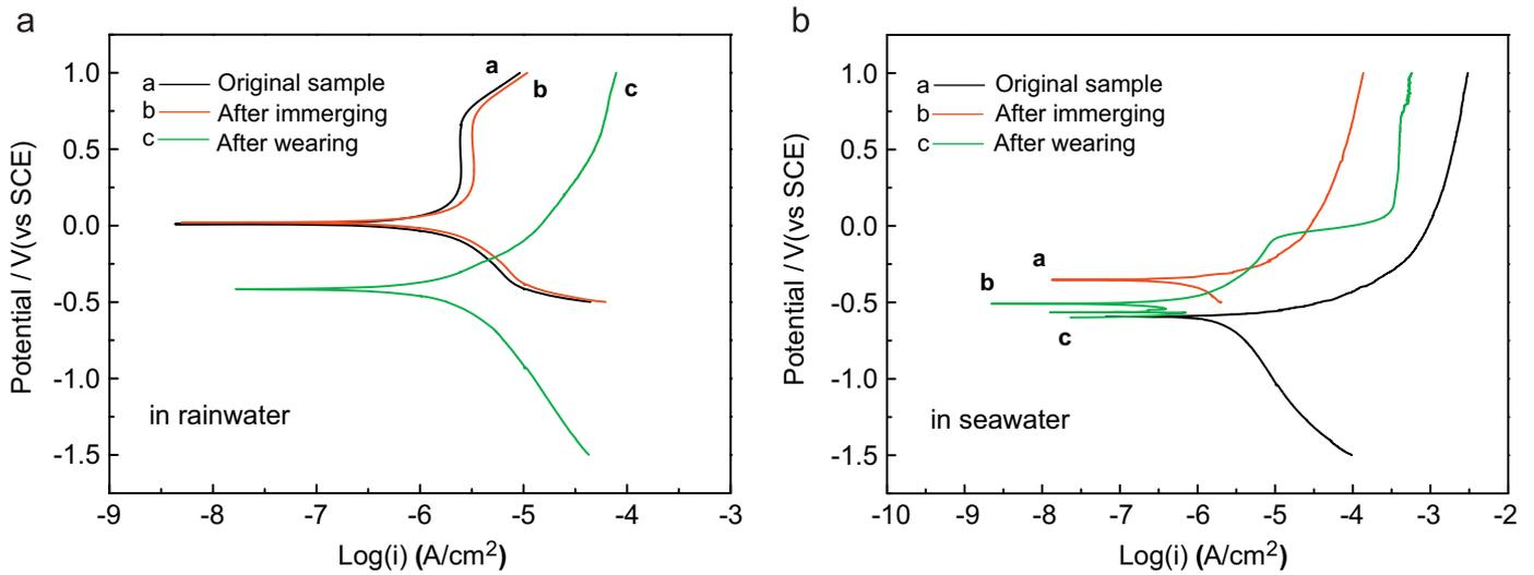
Fig. 9. Polarization curves of MAO Al<sub>2</sub>O<sub>3</sub> coatings with three different states: (a) in rainwater; (b) in seawater.
