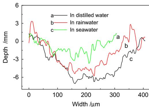
Fig. 8. Profile curves of wear scars in different media at the load of 2 N.
