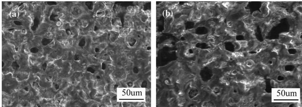
Fig. 5. SEM photographs of MAO Al<sub>2</sub>O<sub>3</sub> coating after immersing in rainwater and seawater: (a) in rainwater; (b) in seawater.
