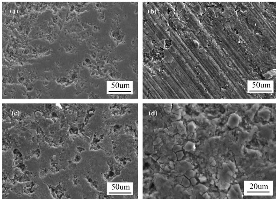
**Fig. 12.** SEM photographs of wear scars in different media: (a) in distilled water; (b) in rainwater; (c) in seawater; (d) a local worn surface in seawater at a larger amplification.
