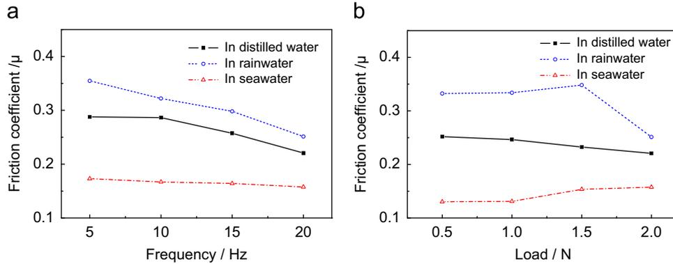
Fig. 6. Friction coefficient in various environments: (a) the frequency versus friction coefficient at the load of 2 N; (b) the load versus friction coefficient at the frequency of 20 Hz.
