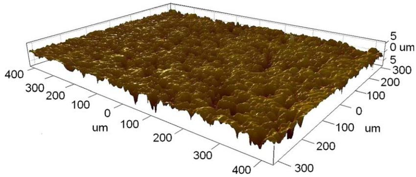
Fig. 4. 3D-image of the MAO coating after polishing.
