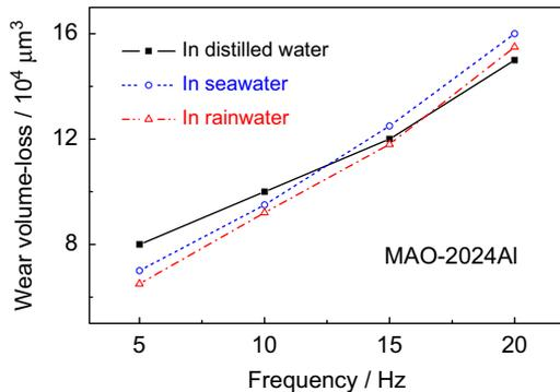
Fig. 7. Wear-loss of the coating under different frequencies at the load of 2 N.
