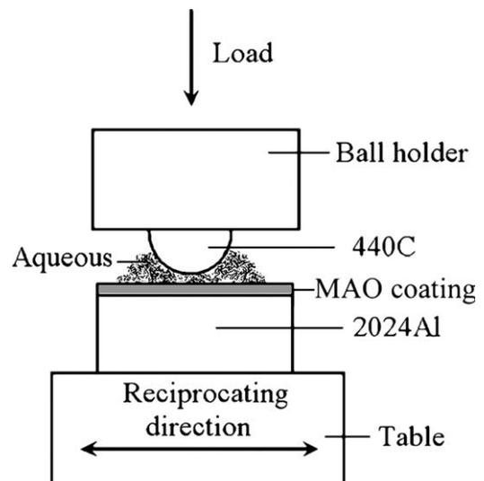
Fig. 1. Schematic diagram of the frictional pair.
