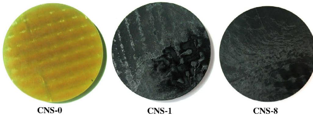
Fig. 2. Original specimens for cone calorimeter test.
