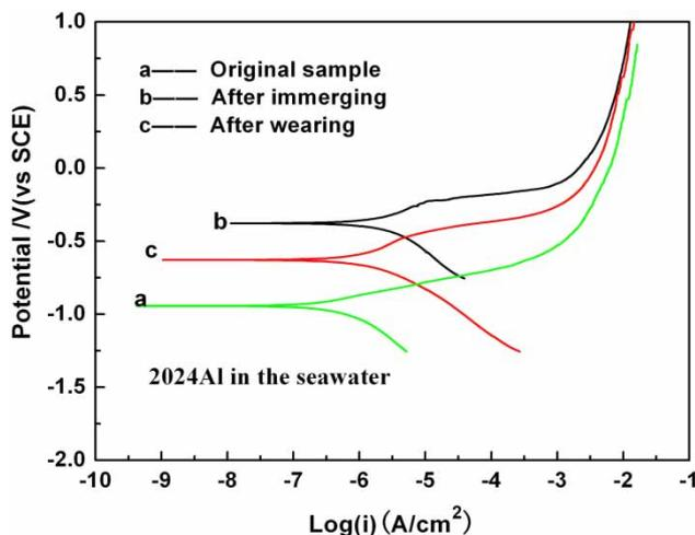
Fig. 3 Polarization curves of 2024Al in seawater
