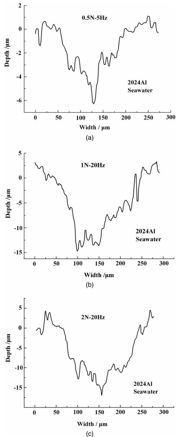
**Fig. 7** Cross-sectional profile curves of wear scars in seawater: (a) at 0.5 N-5 Hz; (b) at 1 N-20 Hz; and (c) at 2 N-20 Hz
