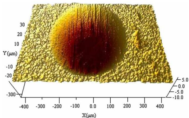
**Fig. 6** Three-dimensional morphology of the cleaned wear scar of 2024Al
