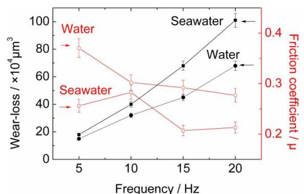
**Fig. 2** Coefficient of friction and wear loss of 2024Al. The dotted line and solid line correspond to the coefficient of friction and wear loss, respectively
