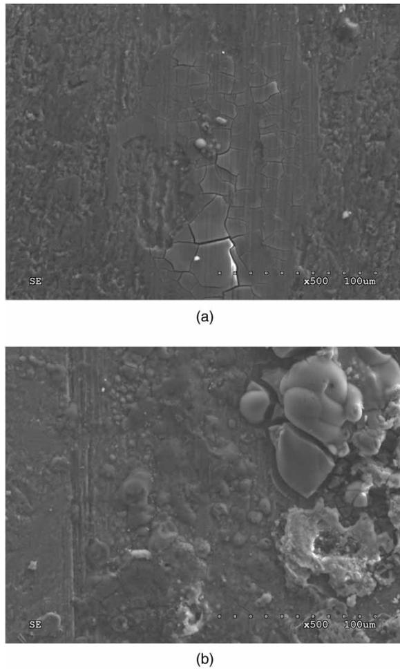
**Fig. 5** SEM photographs of 2024Al wear scars in seawater: (a) at 1 N-10 Hz and (b) at 1.5 N-20 Hz
