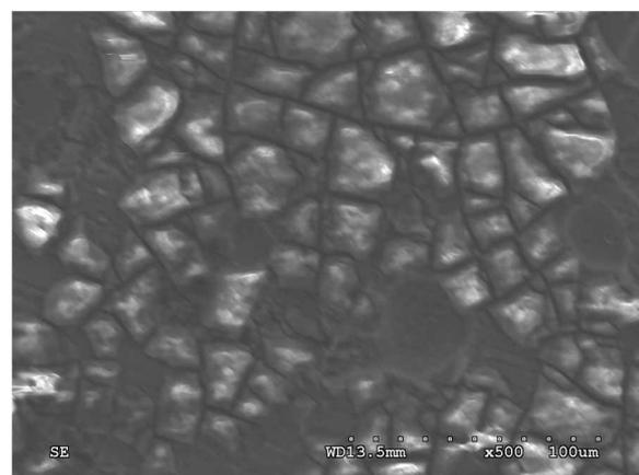
Fig. 4 SEM photograph of the brittle film at the edge of the wear scar of 2024Al in seawater
