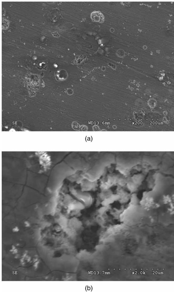
**Fig. 1** SEM photographs of 2024Al aluminium alloy after immersing in seawater: (a) at low-magnification scale and (b) at high-magnification scale
