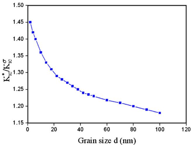
Fig. 5.  $K_{IC}^*/K_{IC}^\sigma$  as a function of grain size  $d$  in nc Ni.
