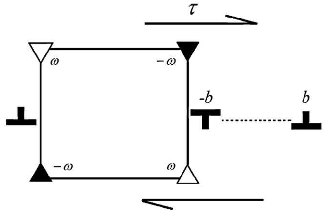
Fig. 3. The transformation from the rotational deformation into plastic shear.
