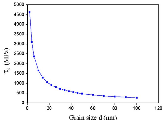
Fig. 4. Dependence of critical shear stress  $\tau_c$  on grain size  $d$  in nc Ni.
