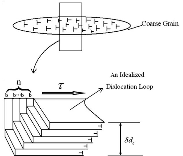
Fig. 3. Arrangement of GNDs within the coarse grain.
