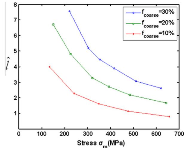
Fig. 7. Variation of nanostructure characteristic length parameter  $\hat{l}$  with  $\sigma_m$  at three different CG contents.
