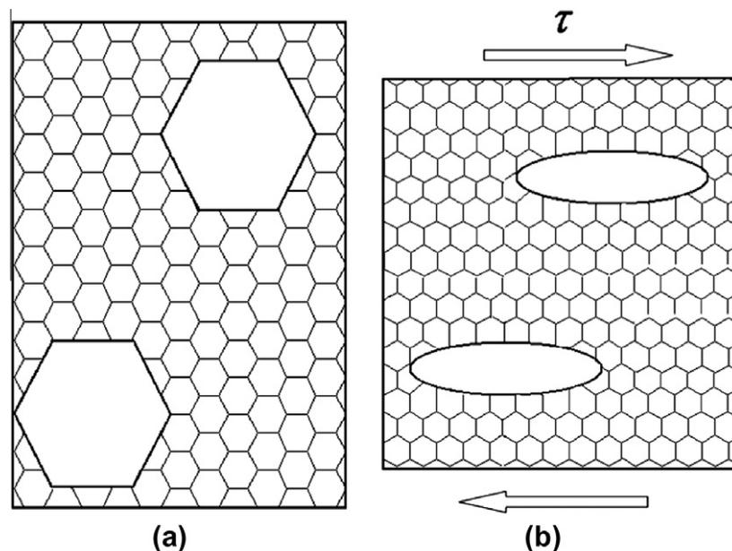
Fig. 1. View of (a) the generated bimodal microstructure and (b) the deformation of the coarse grains when under macroscopical load.
