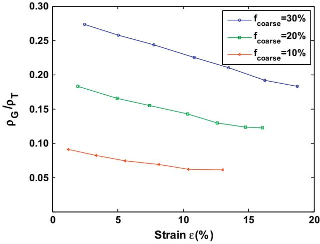
Fig. 5. Ratio of GNDs density to total dislocations density increases with increasing coarse grain content calculated from our model.
