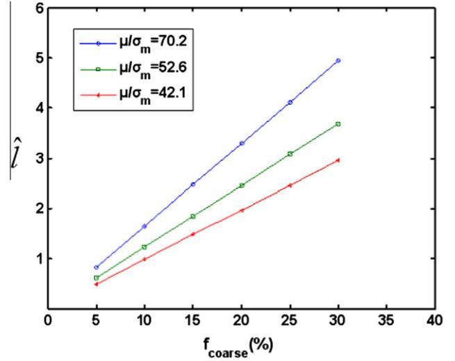
Fig. 6. Variation of nanostructure characteristic length parameter  $\hat{l}$  with  $f_{coarse}$  under three different deformation conditions.
