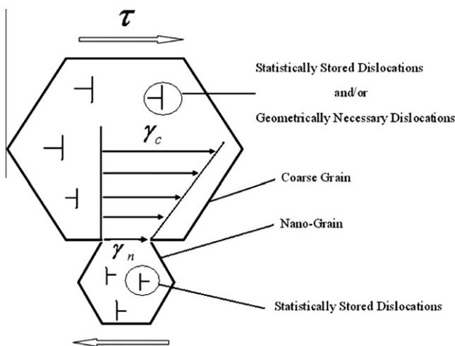
Fig. 2. Two-dimensional composite model undergoes plastic deformation.
