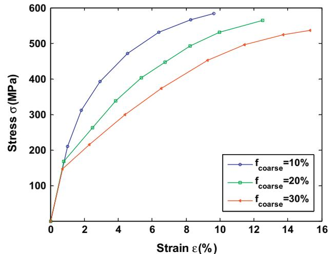
**Fig. 4.** The calculated stress–strain relations (under uniaxial tension) for bimodal nc Cu with different CG contents.
