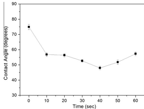
**Fig. 2.** Variation of contact angle as a function of treatment time.
