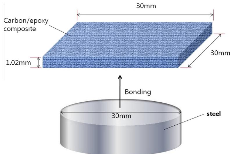
**Fig. 1.** Schematic diagram of wear specimen.
