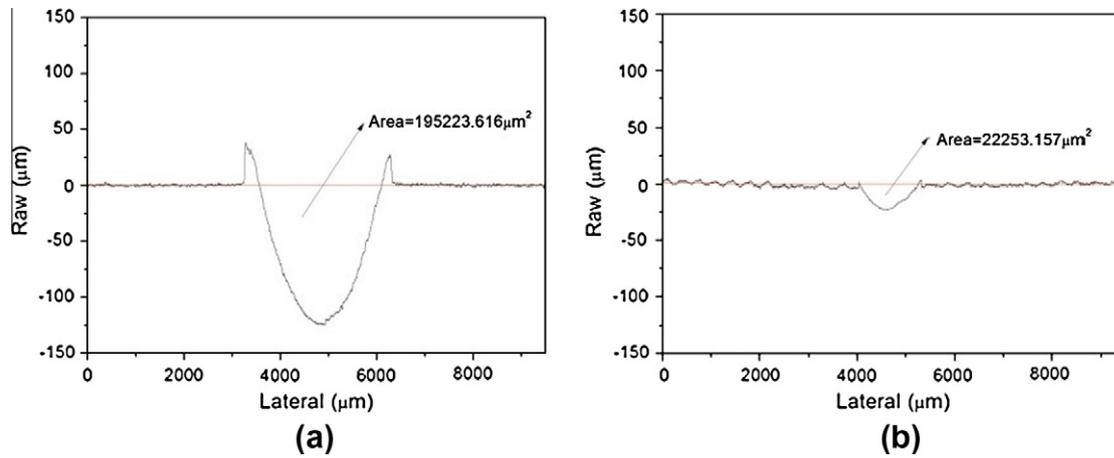
Fig. 6. Variation of depth profile (a) before plasma treatment; (b) after plasma treatment.
