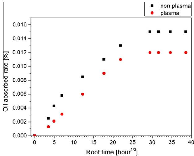
Fig. 3. Oil absorption rate for untreated and plasma-treated carbon/epoxy woven composites as a function of immersion time.
