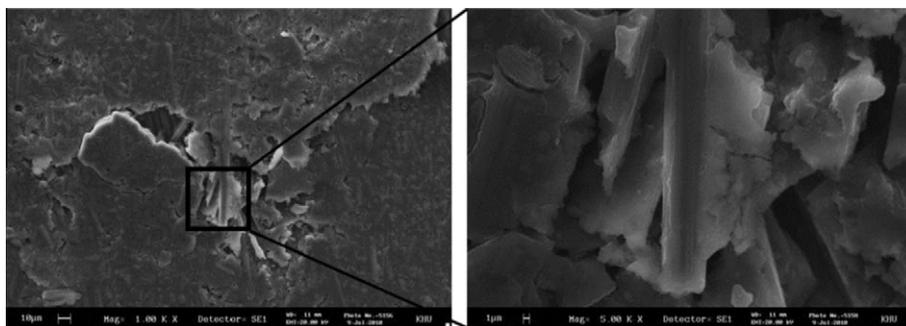
Fig. 9. SEM photographs of worn surfaces of carbon/epoxy woven composites with plasma treatment.
