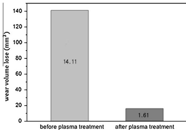
Fig. 7. Wear volume loss of carbon/epoxy woven composites with and without plasma treatment.
