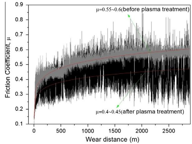
Fig. 5. Variation of friction coefficient of oil-absorbed carbon/epoxy composites with and without plasma treatment.
