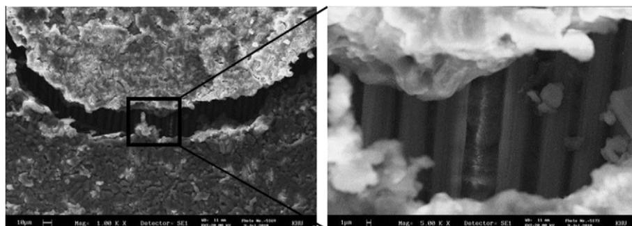
Fig. 8. SEM photographs of worn surfaces of carbon/epoxy woven composites without plasma treatment.
