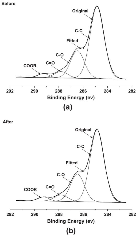
Fig. 4. XPS results of C1s peak with and without plasma treatment (a) before plasma treatment; (b) after plasma treatment.
