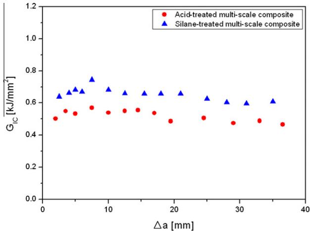
Fig. 8. Comparison of  $G_{Ic}$  values as a function of crack length; (a) acid-treated and (b) silane-treated multi-scale composites.
