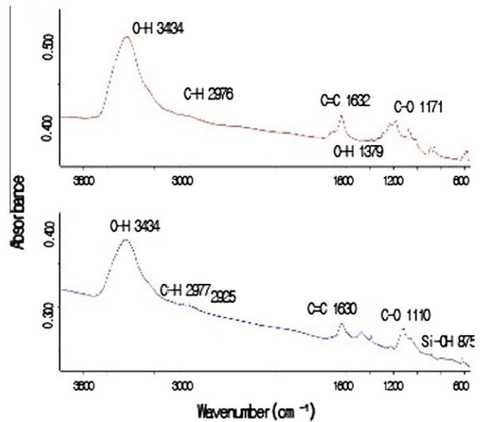
Fig. 2. FT-IR spectrum of (a) acid-treated and (b) silane-treated carbon nanotubes.
