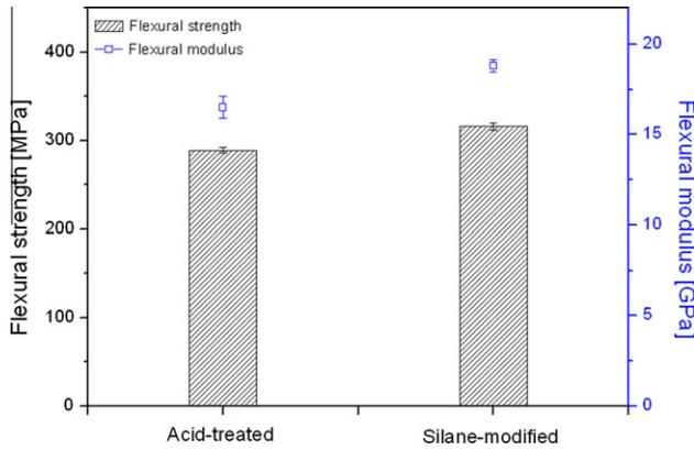
Fig. 4. Comparison of flexural strength and flexural modulus between acid-treated and silane-treated multi-scale composites.
