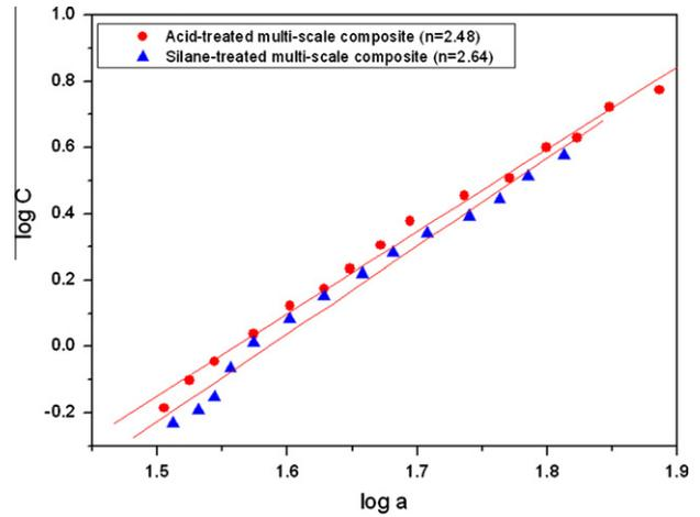
Fig. 6. Comparison of  $n$  values in  $\log C$ – $\log a$  scale.
