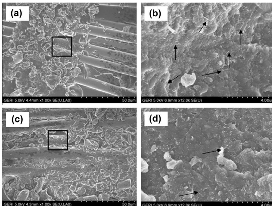
Fig. 9. SEM images of fracture surfaces (a) acid-treated and (c) silane-treated multi-scale composites; (b), (d) are magnified images of boxed region in (a), (c), respectively.
