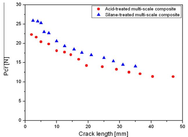
Fig. 7. Comparison of  $P_{cr}$  as a function of crack length.
