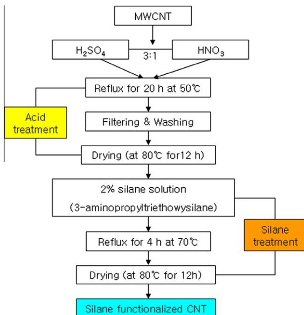
Fig. 1. Flow chart of oxidation and silanization process.
